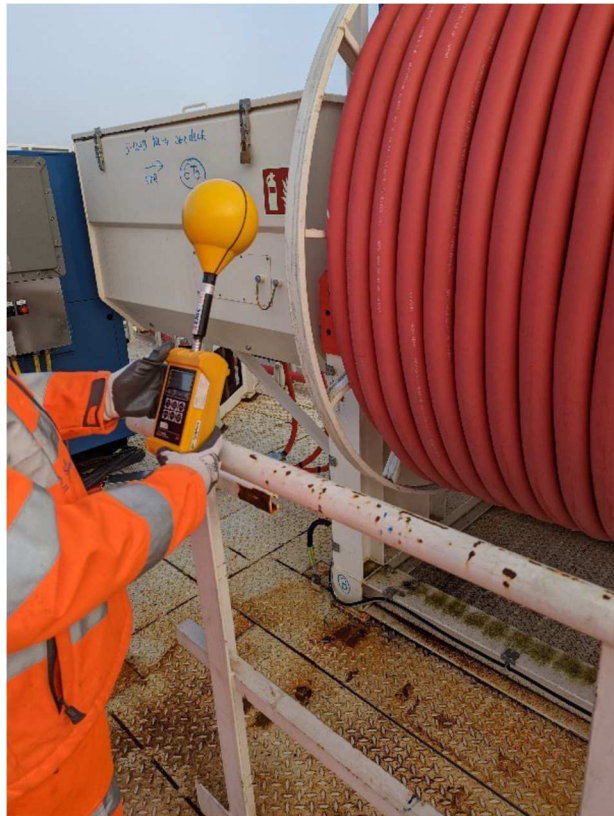
Figure 17 – Example Magnetic Field Measurement Using Hand Held Narda ELT-400 Meter
